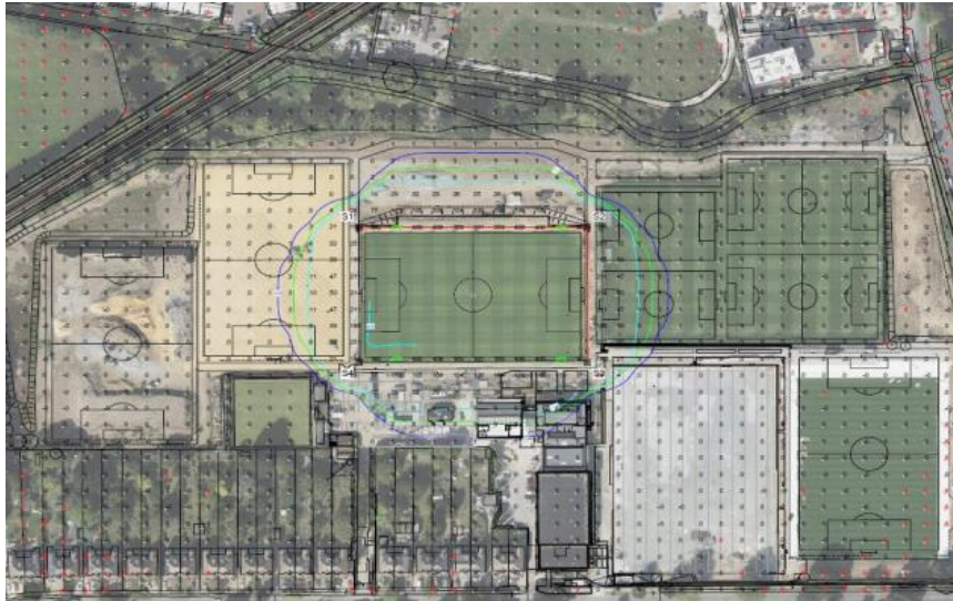
Figure 12 – Image of horizontal light spill contours
